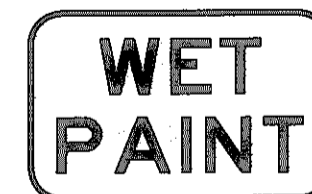
W41-8 SIZE OF SIGN TO BE DETERMINED BY CONSTRAINTS OF STRIPER
